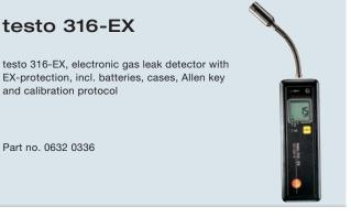
Proof of gas and leakage localization on gas pipes and installations in indoor and outdoor areas The testo 316-EX, which conforms to the guideline 94/9/ EG (ATEX), is a multi-range gas detector with Ex protection for the gases methane, propane and hydrogen. The gas concentrations are measured by the semi-conductor sensor in the ppm range and are shown in the display with a resolution of 1ppm.
