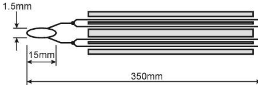
The type R T/Cs had exposed junctions and were each housed in 4mm diameter 2 bore ceramic tube. They were referenced using an Isotech Zeref 136/6 and their outputs were measured using a Solartron 7075 digital multimeter.
