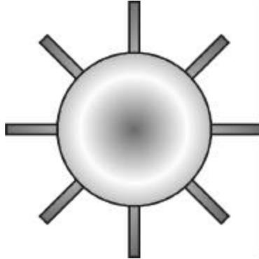
Isotech term this 'the spider'. Spiders can be made to the customer's requirements including having a tube which passes through the ball so that T/Cs with multiple junctions along their length -as used in the semiconductor industry- can be calibrated.
