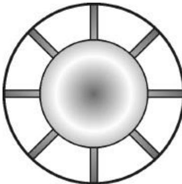
The Saturn that was tested had an 8 legged spider, 4 x 8mm I.D. and 4 x 6mm I.D. The ball had the option of a Platinum foil covering which improves the temperature distribution in the isothermal volume and helps reduce electrical interference which can occur in poorly constructed T/Cs at high temperatures.
