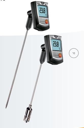
The testo 905-T1 is a particularly fast penetration thermometer with a broad measuring range of -50 to +350 °C, in the short term even up to +500 °C (1 to 2 minutes). The measuring instrument has a professional industrial sensor (thermocouple Type K). It has an excellent level of accuracy, especially in the upper measuring range. The testo 905-T2 is a surface thermometer with a broad measuring range of -50 to+350 °C, in the short term even
