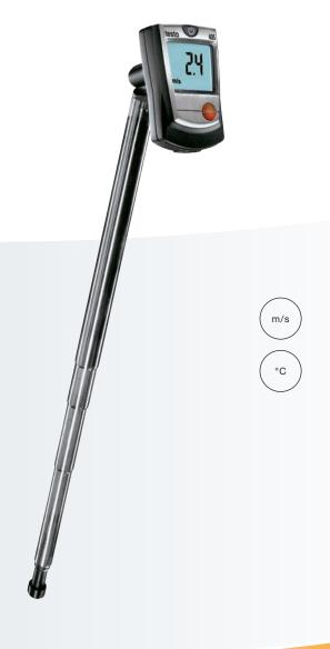
testo 405 is a thermal anemometer. It allows the precise measurement of air flow velocity, volume flow and temperature. With the extendable telescope (up to 300 mm), testo 405 is particularly suited for measuring the flow velocity in ducts. Thanks to the attachment included in delivery, the telescope can be optimally positioned in a duct.
