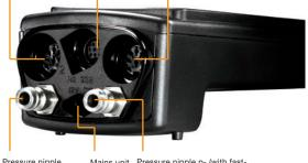
Pressure nipple p+ (with fastaction coupling connection)
