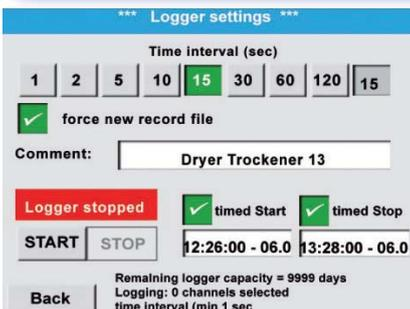
It is possible to store up to 100 million measured values. Each measurement can be stored with a comment, e.g. measuring site name. The time interval can be freely determined.
