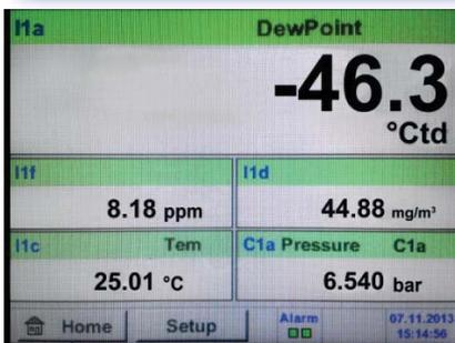
All physical parameters of moisture measurement are calculated automatically. In case of DP 510 the measured values of the third-party sensor are indicated additionally.
