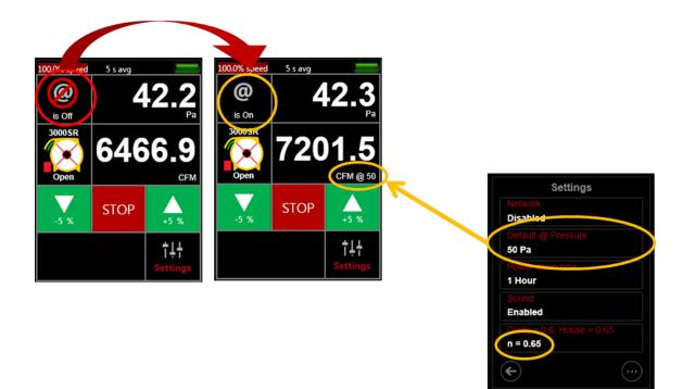
Figure 31: [@ Pressure] extrapolates to "Default @ Pressure" when a speed is set
