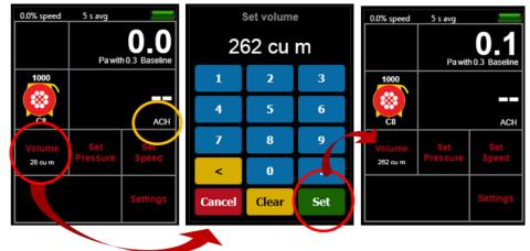
Figure 42: Set [Volume] using metric units when other Results are displayed in metric units
