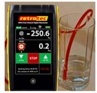
Figure 71: The gauge displaying a negative pressure (-250.6 Pa).
