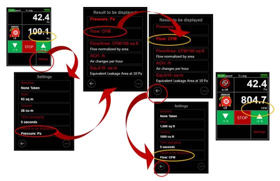
Figure 46: Tap [Settings] to change Result being displayed
