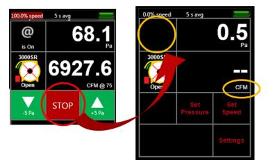
Figure 33: Stopping fan disables and turns [@ Pressure] off
