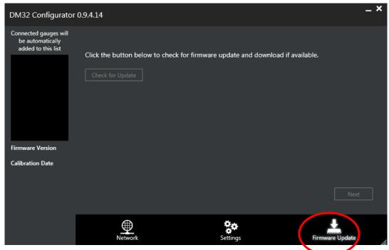
Figure 62: Use Gauge Configurator software to update the firmware in the gauge
