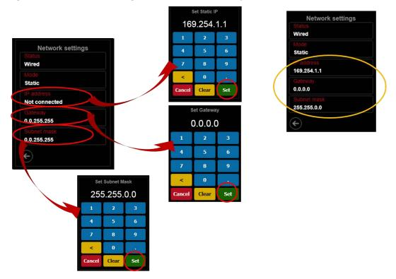
Figure 55: Numeric entry keypads to enter values for "Static" mode Network settings
