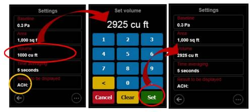
Figure 40: Set the [Volume] needed for ACH Result from [Settings]
