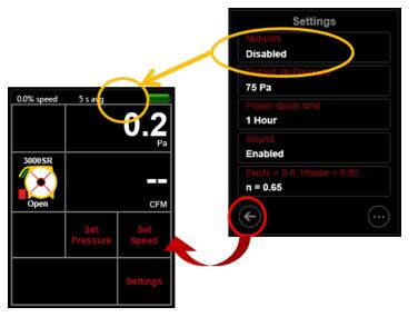
Figure 63: Disable [Network] connection if using USB connection to a computer
