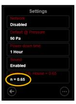
Figure 29: [@ Pressure] extrapolates to the target pressure when a pressure is set
