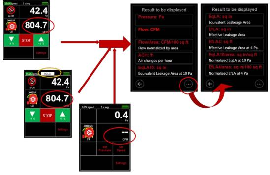
Figure 23: Change "Result to be displayed" during operation
