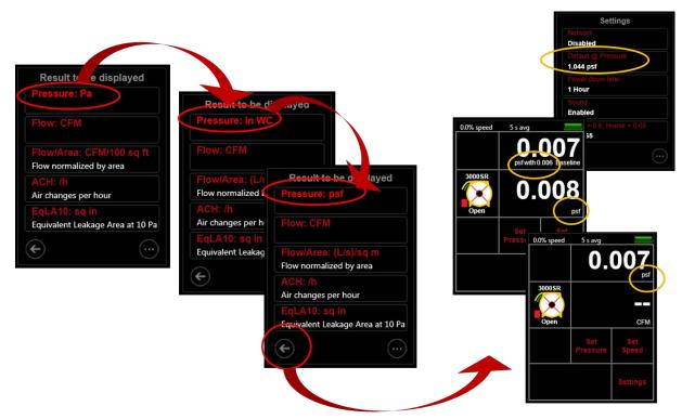
Figure 45: Choose units of Pressure to display (Pa, psf, in WC)
