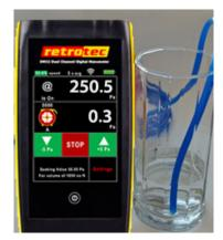
Figure 70: Gauge displaying 250.5 Pa (or 1 in WC).
