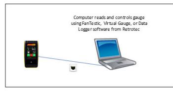
Figure 52: Use "Network" connector to connect a single gauge to a computer
