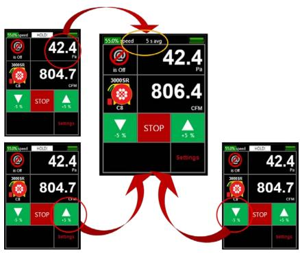
Figure 22: Remove "HOLD!" by tapping [Channel A] or a [Jog] key
