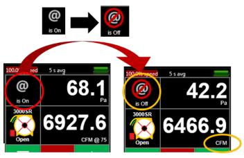
Figure 32: Turn [@ Pressure] off, leaves fan running
