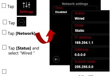
If connecting to Switch or PC, tap [Mode] and select "Static". For 2<sup>nd</sup> gauge enter IP Address: 169.254.1.2
